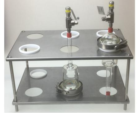
Each type of Amott cell is suitable for both drainage and imbibition tests and custom-made stands are available.
