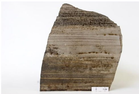
Figure 5. Photograph of hand specimen of oil shale. Note the oil stained parts at top and bottom. Middle part is oil free. Samples OSH and OSV are plugged in the horizontal and vertical direction respectively.
